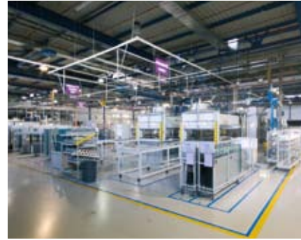
Carrier CO 2 OLtec™ remote cabinet assembly line, Czech Republic
